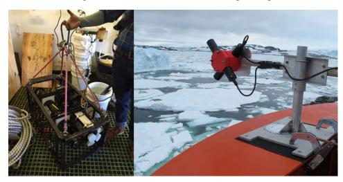
Figure 3. Optical cage (left) and shipborne radiometer (right)
